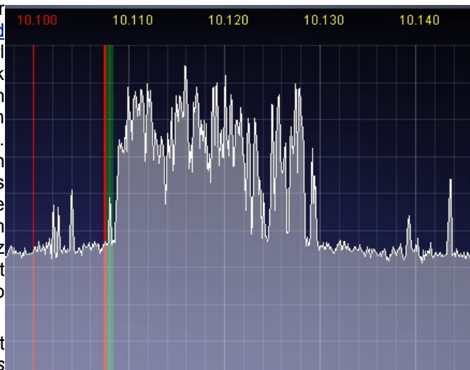
K1N on 30M CW, 10.108 MHz, Jan 3, 00:00UTC. My receiver passband is the green shaded area. Guess he's "listening up!" --AF9A
