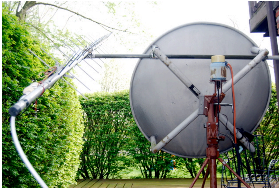
AF9A's antenna setup. The dish isn't used except to hold the 432 MHz antenna (left).
